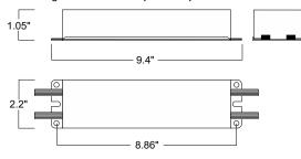
BSL20B6 Battery (dimensions in mm)
