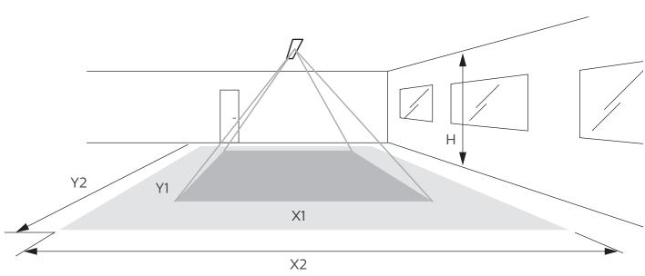
Figure 1. Motion detection area. H: ceiling height. Minor movement detection area: X1 by Y1. Major movement detection area: X2 by Y2.
