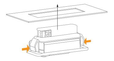
Press springs inwards on both sides before the bracket can slide-in the luminaire hole.
