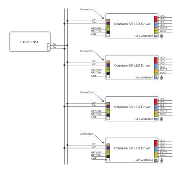
When a group of luminaires is in the same daylight condition and needs to be operated at the same level, it is possible to use one sensor to control multiple luminaires. This can be done in two ways:
