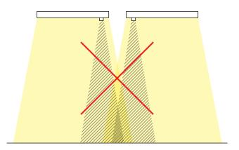
Figure 5. Distance between sensors should be at least 1.5m apart.
